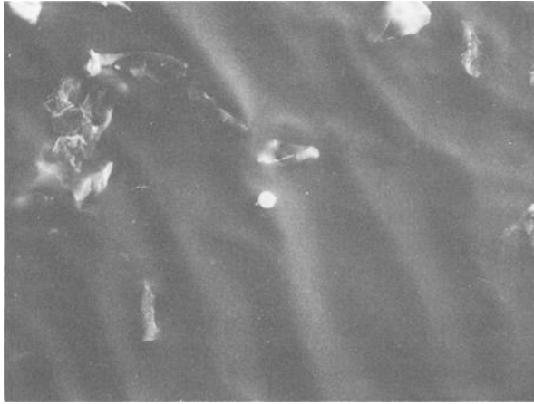
FIG. 2—Typical GSR particle embedded in adhesive tape as seen in the SEM at lower magnification used for searching for GSR on the tape.
